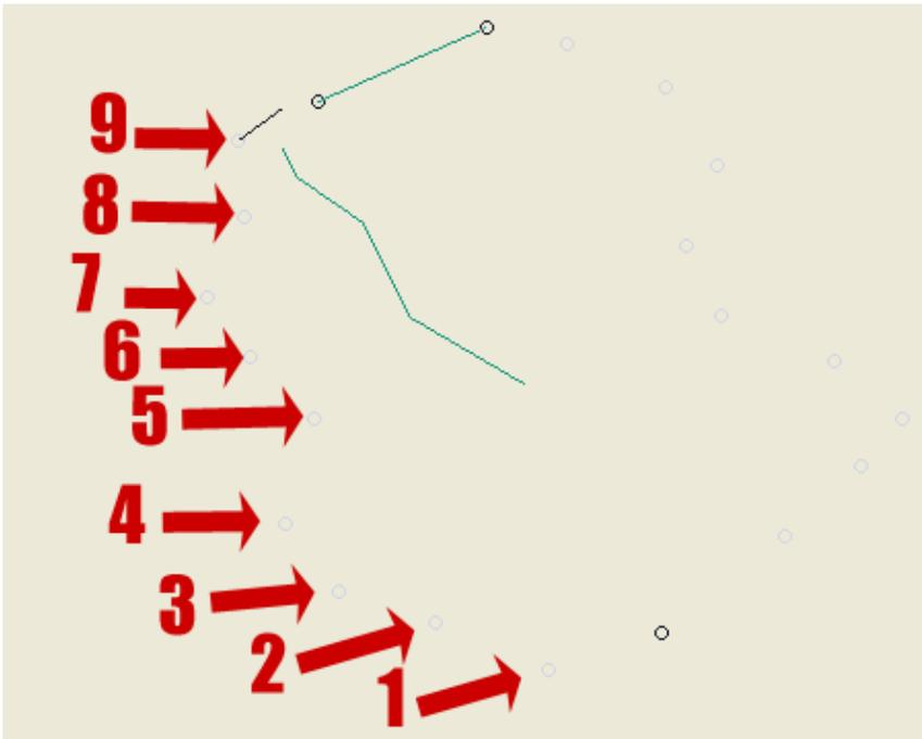
Once the last point is entered which is a run stitch (left mouse button) the complex fill is calculated and created as show below:-
